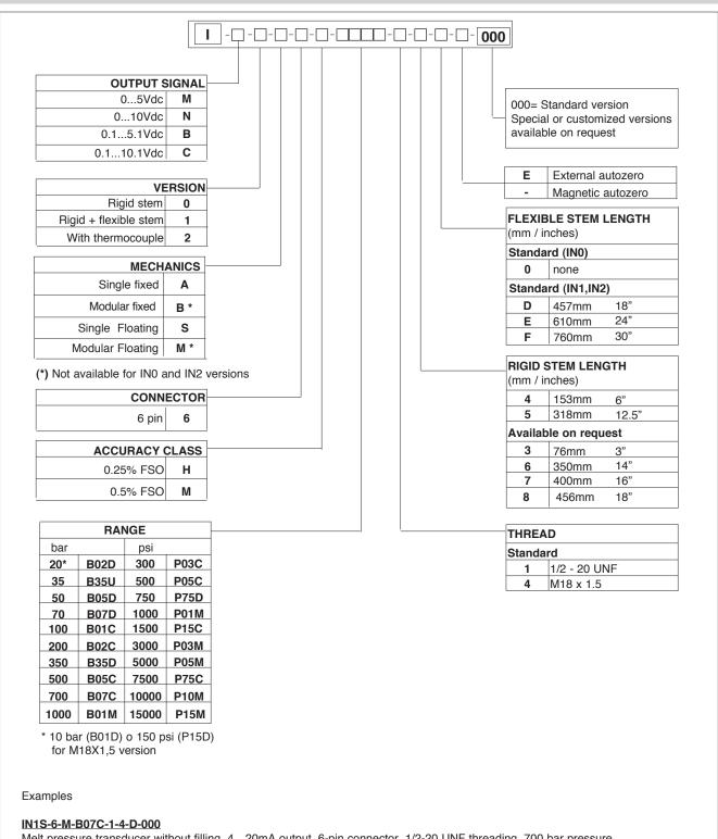
Melt pressure transducer without filling, 4...20mA output, 6-pin connector, 1/2-20 UNF threading, 700 bar pressure range, 0.5% precision level, 153 mm (6") rigid stem, 457 mm (18") flexible stem.
