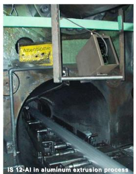
The **IS 12-AI** is a special development of the well proven IS 10-AI for aluminum applications in temperature ranges between 350 and 1050°C.
