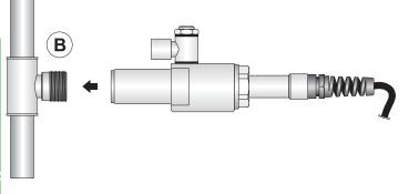
For the connection by treaded coupling, the connection must have an external G 1/4" thread on the side which will be placed in the probe. The connection must be airtight. When installing or removing the probe, it is necessary to depressurize the system.
