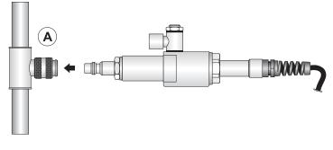
To connect with quick coupling, you can use one of the standard 1/4" couplings provided. Other couplings than those supplied can be used, provided that they have a G 1/4" thread on the side that fits into the probe.
