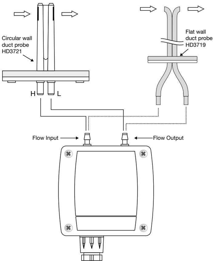
The duct air inlet should be oriented so that the flow enters from the entrance connected to the junction on the left in the container leaving from the right one.
