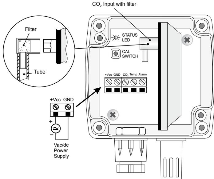
Open the instrument top cover to discover the CAL SWITCH calibration key on the board and the calibration gas inlet.
