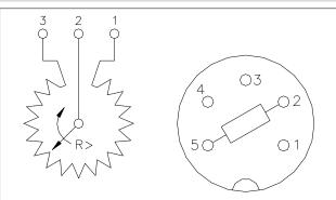
A  $5\mbox{K}\Omega$  protection resistance has been connected between pins 2 (cursor) and 5; in case of the cursor is connected to pin 5, eventual short-circuits due to wiring errors are avoided.
