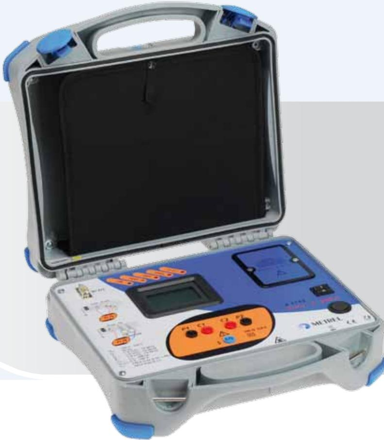
The **Euro - Z 290 A** is a professional portable test instrument intended for **low impedance measurements** in environments up to **CAT IV /310 V**. It can operate alone or in combination with the METREL instruments. **High precision line impedance** and **high precision fault loop impedance** measurements in range from 1 m $\Omega$  up to 19.99  $\Omega$  are its excellence.
