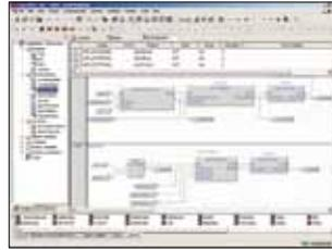
The basic idea behind PLC programming with the function block diagram is that the program is structured in function-oriented logical sequence cascades (networks). FBD derives from the graphic representation of flow diagrams, hence its ease of use.
