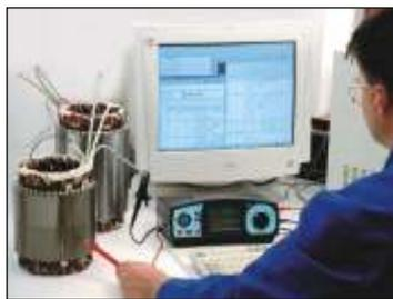
Diagnostic test of motor windings
