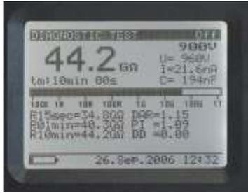
Large custom LCD dot matrix display with bar graph and with back light. Simultaneous display of measurement parameters. Built-in timer and real time clock.
