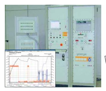
voltages, currents, outputs, energies, temperatures, rpm and direction of rotation, water consumption and water pressures can be acquired, recorded and analysed in concrete figures.
