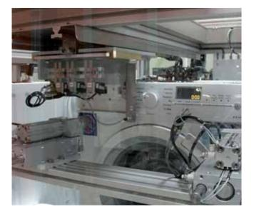
This is because controlled adaptation of the devices is indispensable for smooth serial production. On the one hand, there is the requirement to adapt the test pieces with the voltage supply and water and waste water connections; on the other hand,
