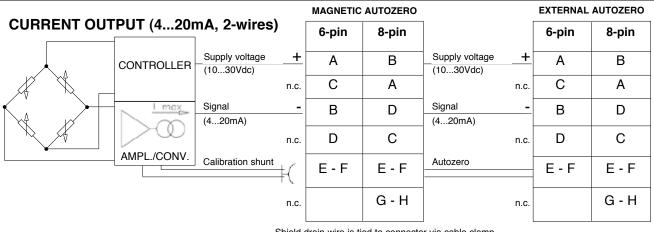
Shield drain wire is tied to connector via cable clamp
