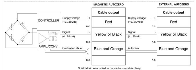
8 pin connector PC02E-12-8P **Bendix**
