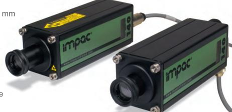
The **IN 140/5** is a digital pyrometer for non-contact temperature measurement of glass and quartz glass surfaces with temperature ranges between 250 and 2500°C.
