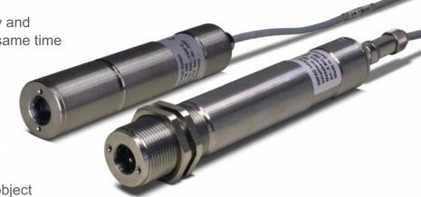
The IS 300, IS 310, IGA 300 and IGA 310 are stationary pyrometers for non-contact temperature measurement of metallic surfaces, graphite, ceramics, etc.
