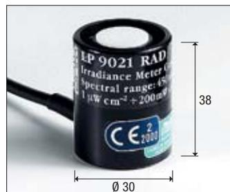
**LP 9021 RAD:** Radiometric probe for measuring the **IRRADIANCE** of artificial light sources, irradiance of the sun.
