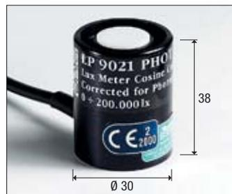
**LP 9021 PHOT:** Photometric probe for measuring **ILLUMINANCE**; photopic filter in compliance with CIE n° 69 - UNI 11142, diffuser for correction according to the cosine law.
