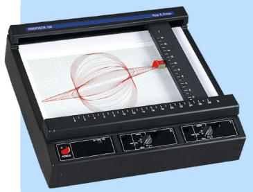
The SERVOGOR 790 is a potentiometer recorder in DIN A4 version, which records the functional dependence of two DC voltages Y = f(X) in perpendicular coordinates or, with the help of the integrated time unit, a DC voltage as a function of time Y = f(t)
