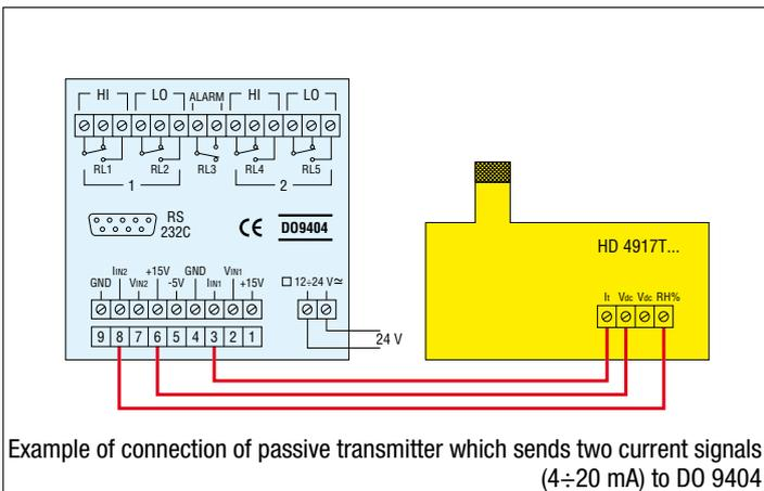
Example of connection of passive transmitter which sends two current signals (4÷20 mA) to DO 9404
