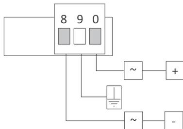
Fuse - To comply with security regulation 61010-1, add to the power line a protection fuse acting as disconnection element, easily accessible to the operator and identified as a protection device.
