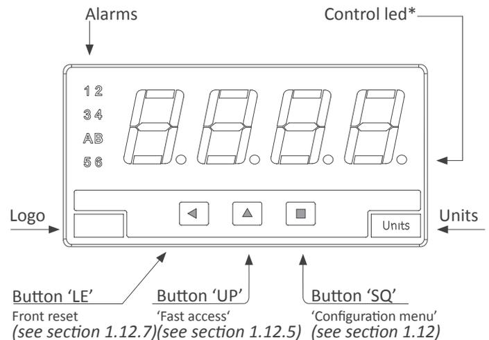
\* The 'led control' is operative only in counting modes that do not display seconds or tenths of second. It flashes 'on' and 'off' at a rate of 1 second when instrument is counting ('start'). It remains 'off' when the instrument is not counting ('stop').
