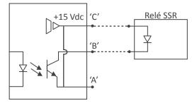
Schematic for SSR control module
