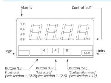
\* The 'led control' is operative only in counting modes that do not display seconds or tenths of second. It flashes 'on' and 'off' at a rate of 1 second when instrument is counting ('start'). It remains 'off' when the instrument is not counting ('stop').
