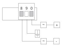
Fuse - To comply with security regulation 61010-1, add to the power line a protection fuse acting as disconnection element, easily accessible to the operator and identified as a protection device.
