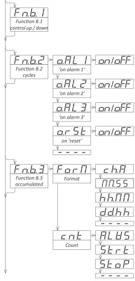
• the 'State' ('StAt') parameter controls the state of the counter after power-up. Select 'Strt' to count after power-up or 'StoP' to remain stopped after power-up.
