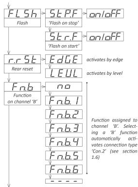
Next menu entry gives access to the configuration parameters of the 'channel 'B' function' ('Fn.b') previously selected. If no function has been selected, menu entry indicates 'Fn.b.n'. Following is an explanation for menus 'Fn.b.1' to 'Fn.b.6'.
