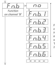
Function assigned to channel 'B'. Selecting a 'B' function automatically activates connection type 'Con.2' (see section
