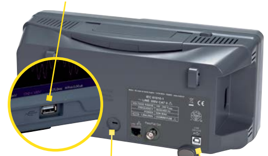
Provided with a built-in Kensington anti-theft system USB port for communicating with a PC
