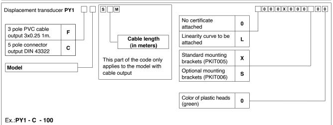
Displacement transducer model PY1, 5-pole connector output, useful electrical stroke (C.E.U.) 100mm.
