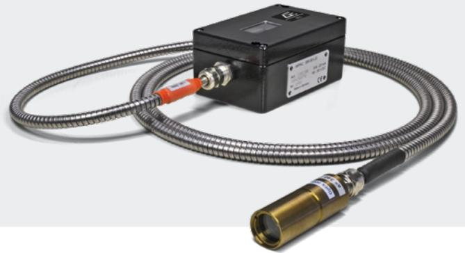
The Impac® ISR 50-LO digital, highly is an accurate two-color pyrometer with fiber optic for non-contact temperature measurements in temperature ranges between 700 and 3000°C. The instrument is equipped with an optical fiber, which can be used in very high ambient temperatures up to 250°C without cooling and it is unaffected by electromagnetic interferences.
