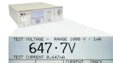
With the introduction of 17th Edition regulations, the minimum insulation resistance values have been changed from the 16th Edition requirements. The 3200 provides compliance to both sets of regulations, with 16th and 17th Edition modes available at the press of a button.
