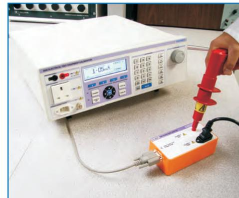
The flash test option provides a safe and easy method for measuring PAT flash voltage and current at Class 1 and Class 2 settings.
