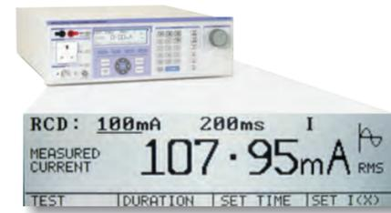
RMS and Peak current measurements for all types of tester using digital waveform capture & analysis.
