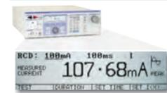
Accurate & repeatable trip times entered simply via the keyboard provide easy calibration.
