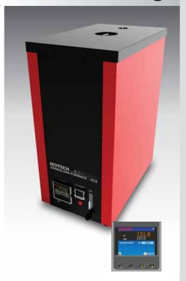
drive. The PID control parameters are now dynamically optimised at different temperatures optimizing furnace stability.
