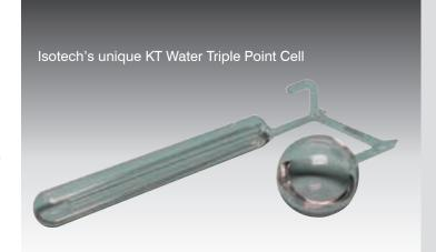
Reverting to the very first designs of water triple point cells, Isotech produce a cell with Isotopic analysis, a McLeod gauge to assess any trapped air and an attached flask where the cell's water can be transferred and redistilled. By accounting for these sources of uncertainty we claim that this cell represents the ultimate reference for those requiring cells as close to ITS-90 as possible. Please ask for a copy of a comprehensive report describing the cell, its operation and performance.
