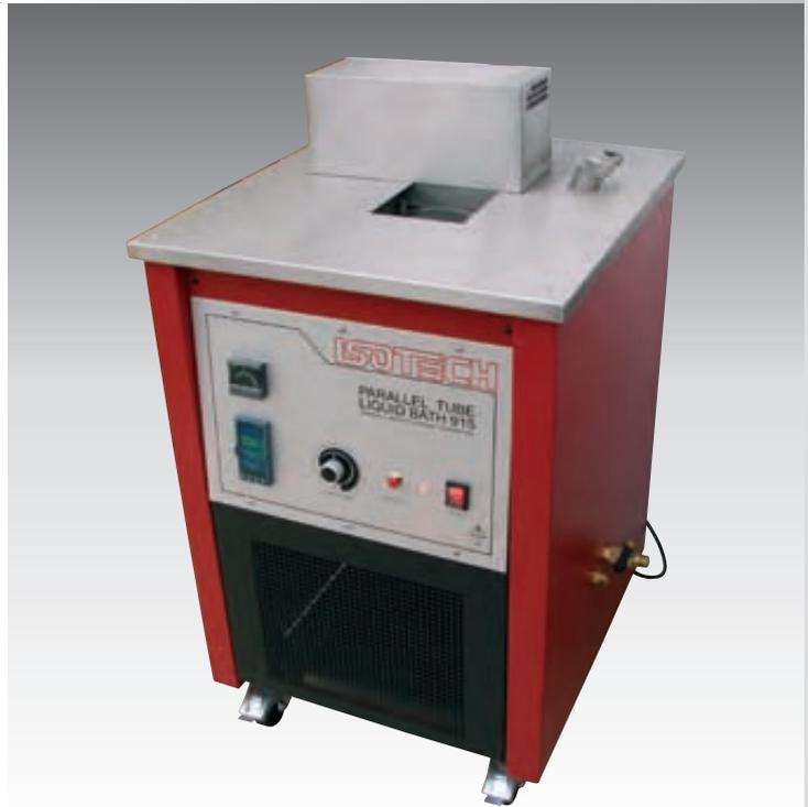
The standard temperature controller has resolution from 0.01°C to 0.1°C which auto scales to suit the four digit display (all digits can be read with the Cal NotePad Software).
