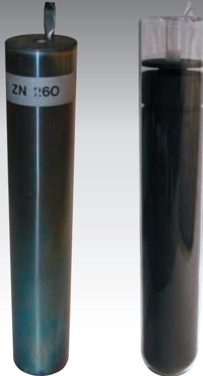
Cost effective dedicated desktop apparatus like the POTTS, "Points on the Temperature Scale" can be used to automatically bring the cell to the plateau. These simple to use systems conveniently provide long flat plateau for low uncertainty calibration of thermometers.
