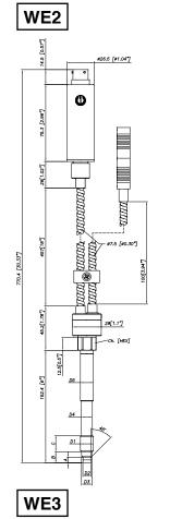
14.5 [0.577] ø26.5 [ø1.04"] Exposed capillary **(** D1 1/2-20UNF 75.3 [2.967] .307/.305" D2 [7.80/7.75mm] D3 .414/.412" [10.52/10.46mm] .125/.120" [3.18/3.05mm] 810.8 [31.97] .318/.312" [8.08/7.92mm] .81" 440[17.32"] [20.6mm] ø9[0.35"] ø1.6[0.06"] 15[0.59"] 240 [9,47]
