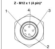
Every connector has a protection rating IP69K/IP67 with female connector properly installed. M12 with female homologated connector mounted, tightening torque 0.6Nm + low strenght threadlocker
