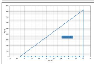
The diagram shows the optimum ratio between load and power supply for transmitters with 4...20mA output. For correct function, use a combination of load resistance and voltage that falls within the two lines in the graph above.
